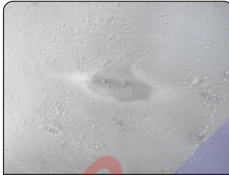
Photo 137: Keel exposed and rusting Bottom paint peeling
