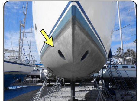
Photo 94: Bow thruster tube is off center line of vessel (Slightly forward on starboard side)
