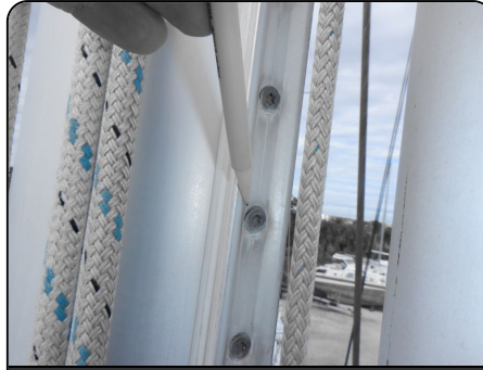
Photo 43: Screws backing out of top of track
