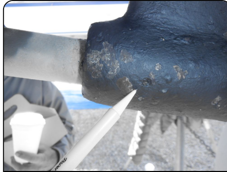
Photo 124: Cutless Bearing set screws in place
