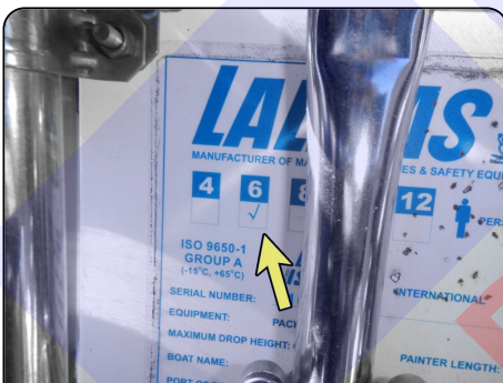
Photo 16: 6 person Life raft Needs Re-certified
