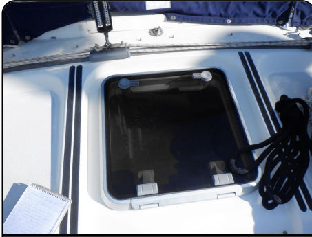
Photo 27: Salon escape hatch
