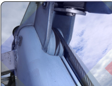
Photo 54: Shives at the top of the mast
